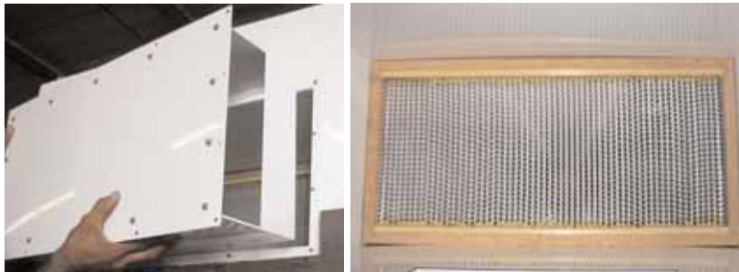
5.1 Replacing the Purge Module HEPA Filter. Remove the #10 cap nuts for filter access
